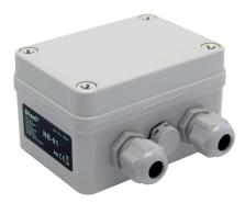
**Non-hermetic junction box NB** is used for termination of a cable with compensation tube and electrical connection to supply cable. The connection is provided using a terminal block inside the box. The junction box contains a membrane for ingress of atmospheric pressure and protection against ingress of moisture. The NB box is primarily intended for connection of hydrostatic level meters HLM-25C, HLM-25S, HLM-16N, HLM-35C and HLM-35S.
