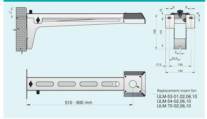
\* The distance of the holes from the upper edge of the wall should be chosen with regard to the material and its quality.
