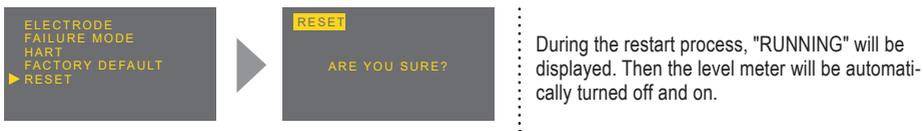
During the restart process, "RUNNING" will be displayed. Then the level meter will be automatically turned off and on.
