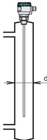
E - electrode length [mm] – select so that the electrode end is submerged at least 20 mm below the lowest measured level
