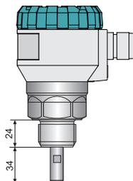
Fig. 10: The level meter without an electrode
