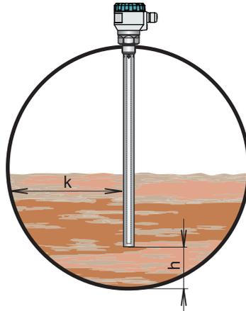
**h** - distance from the bottom – at least 50 mm due to the possible presence of heavier fractions (water) in petroleum products
