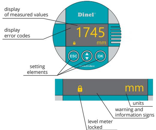
\* flashes intermittently when receiving a reflected signal (echo) from the measured level
