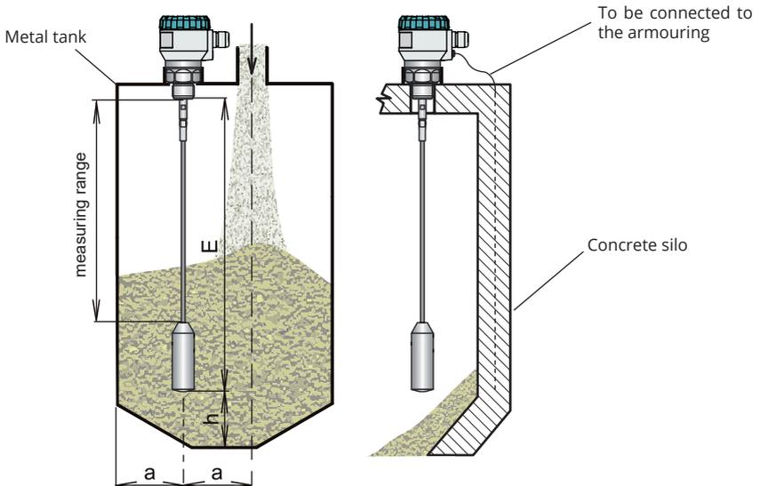
**E** - electrode length [mm] – to be selected so that the electrode end is placed at least 20 mm below the lowest measured level
