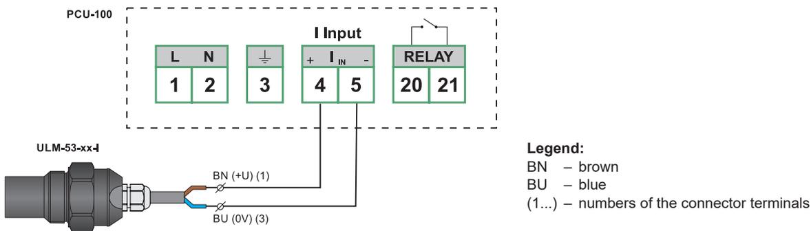
*The level transmitter ULM-53-XX-I may be replaced by any other sensor with current output.*
