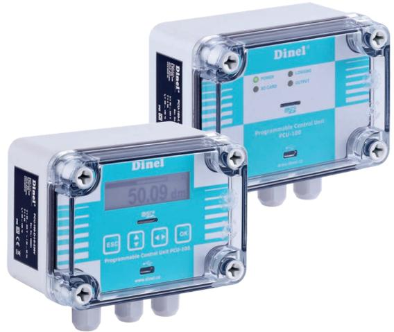
**Programmable control unit PCU-100** is used for measurement, displaying and archiving of the physical value (liquid level, pressure, flow, temperature, etc.). One transducer of physical magnitude with an analogue 4-20 mA output can be connected to the unit.
