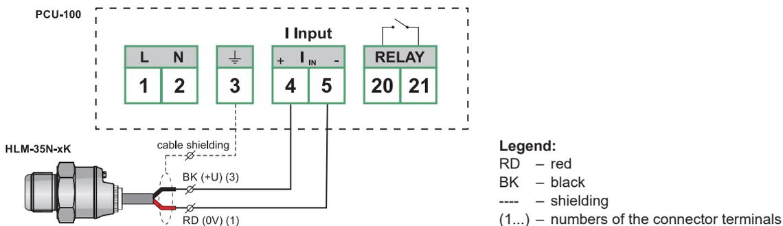
**Example of wiring several HART-enabled level meters:**
