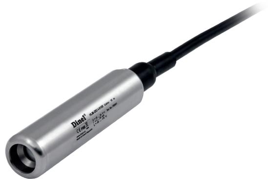
**Hydrostatic level meter HLM-25C** is compact measuring device containing ceramic tensometric sensor and evaluation electronics in stainless steel probe. Ceramic sensor is resistant to lightly soiled, or sludge water. From the probe housing comes out 2-wire cable with capillary (for atmospheric pressure compensation). The front side of the sensor is open, therefore the level meter is resistant to capture gross (solid) impurities. The level meter has no customer-accessible adjusting elements.
