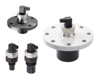
**Ultrasonic level meters ULM**® is self contained device, that includes electroacoustics transducer and electronic module. The level meter ULM transmits series of ultrasonic pulses, which propagates towards the liquid surface. Reflected acoustic wave is received back in the ULM transducer and processed in electronic module. The distance calculations are based on time of flight of the acoustic wave to the level and back.
