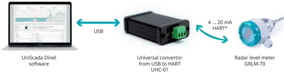
Fig. 47: Connection of peripheral devices by HART® communication protocol using UHC-01
