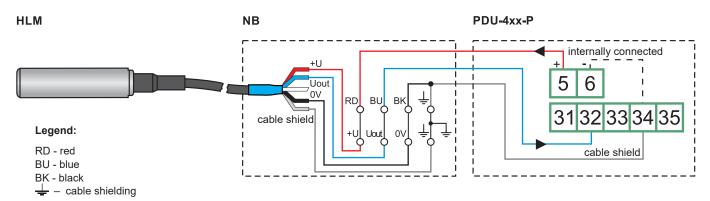
If junction box with integrated overvoltage protection is used, the sensor must be connected to the bottom contacts of the terminal block. These contacts are identified with SENSOR label.
