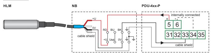
If junction box with integrated overvoltage protection is used, the sensor must be connected to the bottom contacts of the terminal block. These contacts are identified with SENSOR label.
