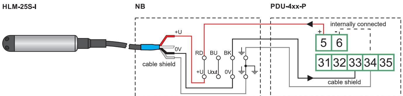
In the case using a connection box with integrated overvoltage protection, the sensor needs to be connected to the bottom series of terminals. This series of contacts is marked by label SENSOR.
