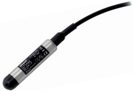
**Hydrostatic level meter HLM-25S** is compact measuring device containing silicon strain gauge sensor and evaluation electronics in stainless steel probe. From the probe housing comes out 2-wire cable with capillary (for atmospheric pressure compensation). The front side of the sensor is equipped with plastic removable cap (to avoid membrane damage). The level meter has no customer-accessible adjusting elements.
