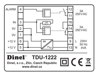
Symbol of producer: logo Dinel<sup>®</sup> Internet address: www.dinel.cz Country of origin: Made in Czech Republic Double insulation sign (equipment protection class II.): □ Compliance mark: **C** Electro-waste take-back system mark: X Block and wiring diagram.
