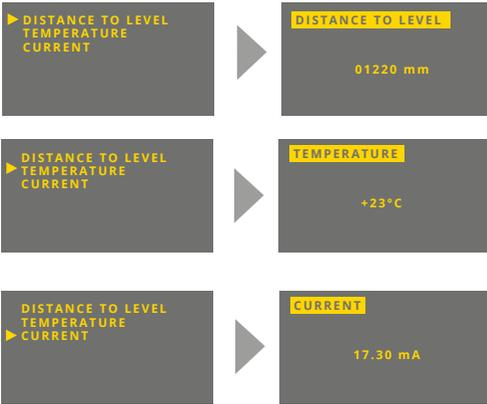
The temperature is measured inside the tank where the level meter is installed.
