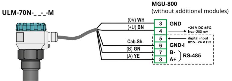
8.5. WIRING DIAGRAM OF THE LEVEL METER WITH MODBUS / RS485 AND PDU UNIT
