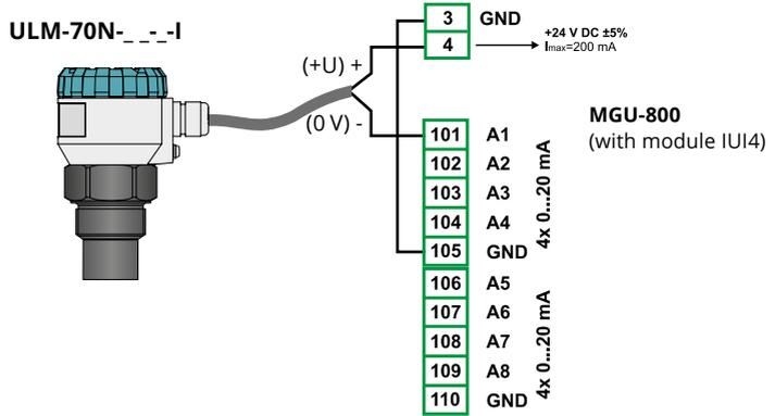
8.4. WIRING DIAGRAM OF THE LEVEL METER WITH MODBUS / RS485 AND MGU UNIT
