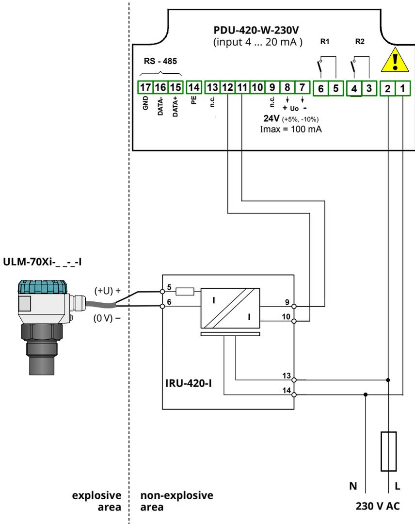
**i** Connection of PDU-420-W is valid for firmware version 6.00 or higher. The older versions (up to version 5.99), the terminal 9 of the IRU unit is connected to the terminal 10 of the PDU unit and the terminal 10 of the IRU unit is connected to the terminal 11 of the PDU unit.
