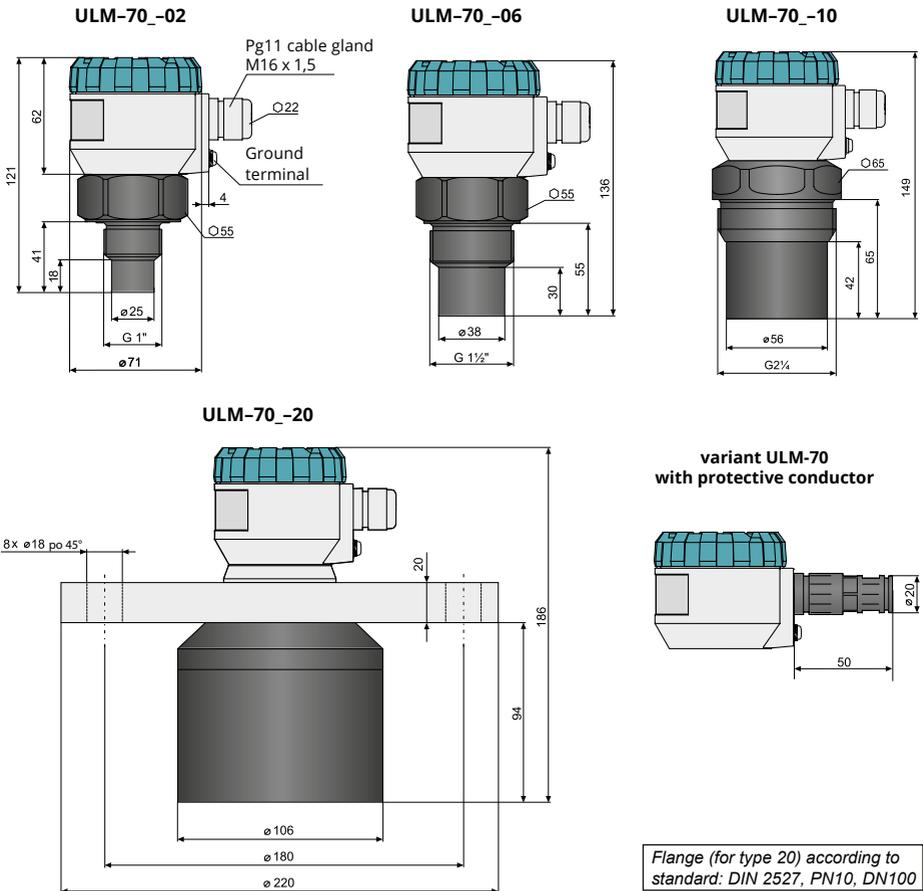
Flange (for type 20) according to standard: DIN 2527, PN10, DN100
