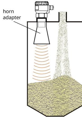
Fig. 8: Level meter installation in silo or hopper
