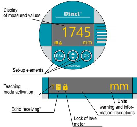
\* Slow flashing while the reflected signal (echo) is received from the measured level.
