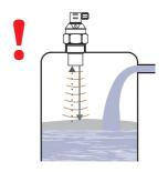
Fig. 5: Thick foam on the surface
