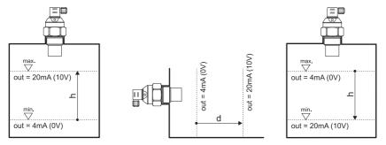
Fig. 18: Basic mode (measurement of level height)
