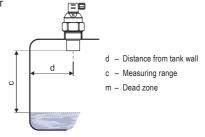
Fig. 3: Installation distance from the tank wall
