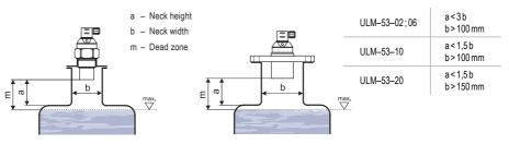
Fig. 4: Possible installation of the installation neck
