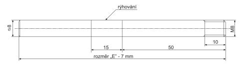
Fig. 15: Drawing of the measuring electrode with marked thread for connection and grooving
