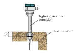
Fig. 6: Installation of the level meter in an insulated tank
