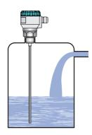
Fig. 8: Installation of the level meter out of the reach of filling flow
