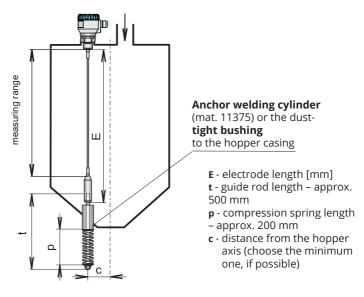
Fig. 4: Installation of the level meter with a rope electrode and anchor
