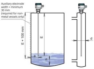
Fig. 1: Installation of level meters with rod electrodes
