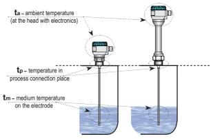
Fig. 19: Illustration of temperature measurement areas
