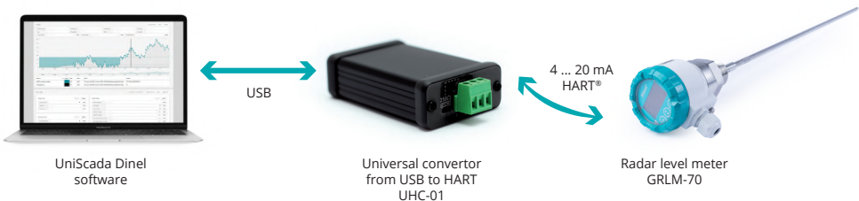
Fig. 49: Connection of peripheral devices by HART® communication protocol using UHC-01
