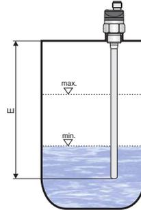
Fig. 4: Two state regulation by hysteresis setting
