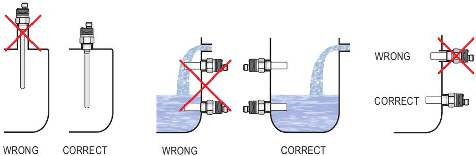
Fig. 5: Long fitting tubes in side wall mounting
