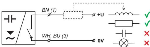
Fig. 7b: "S" type sensors connection
